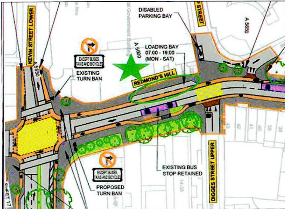
Figure 2: Extract from General Arrangement Aungier Street drawing (Tesco Express store indicated by star)
